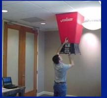
Flow hoods: provide 'real-time' and actual airflow volumes from duct registers
