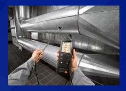
Traverse reading airflows through ductwork
